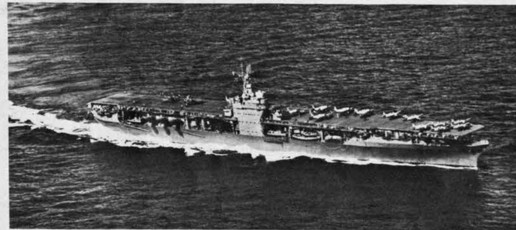
OLDEST U. S. KEEL-UP CV is the Ranger. Unlike our other big carriers, she has her stacks separated from small rectilinear island. Three stacks project from each side in the aft quarter.
